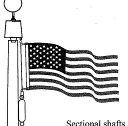
GENERAL: CONCORD Independence winch-type concealed halyard flagpoles are made from all new seamless 6063-T6 aluminum tubing, having a uniform conical taper of approximately 1" in every 5'6". Overall lengths to 38'6" can be fabricated in one piece. Overall assembled lengths of 28'0" to 38'6" can be fabricated in two sections for easier shipping. Assembled lengths of 44' & 49'6" are produced in 2 sections. Assembled lengths of 55' to 88' are produced in 3 sections.
